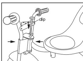
3. Insert the front main frame into the front fork, then lock them with the clip, pushing it till the end.
