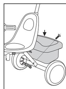
8. Push the basket hardly, get it stuck on the iron tube of the end of the main frame, then lock it with screw and put.
