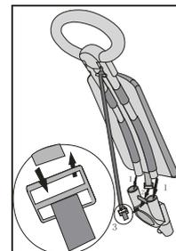
6. Insert the two handlebar tube into the two holes on the plastic connector, then pull the buckle through the plastic connector. Finally insert the belt through the buckle.
