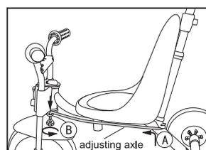
4. Put the adjusting axle through the A and B, lock them with nut.
