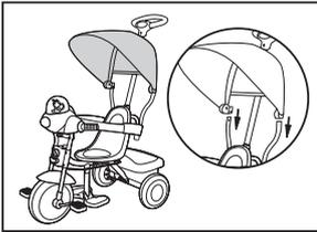
13. Insert the canopy connector into its fixing block, then canopy fixed after the two poles spring card out from canopy block.
