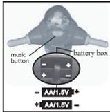
Music: Open the cover of the battery box on the head part, and put in two battery (size AA). Close the cover, and the push the button to play the music.
