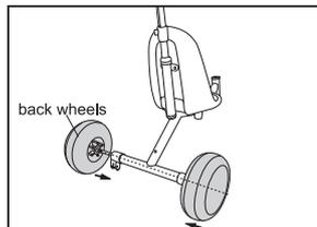
2. Insert the rear wheels axle into the axle's linking tube, and then insert the axle into the hole of wheels.
