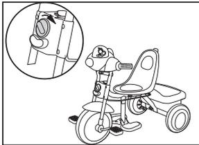
12. Adjusting: Turn the directional knob on the front of the tricycle's body to change the way of the tricycle (going straightly or changing direction)
