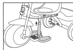
10. Insert the footrest into the main frame till it locked.
