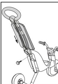
7. Insert the pushing handlebar into the adjusting tube (down) and tight it with screw. Adjusting the height of the handlebar: release the screw, move it upward or downward till the right place and then tight the screw.
